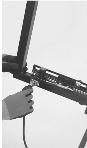
7. Connect Power Cable to Bow
