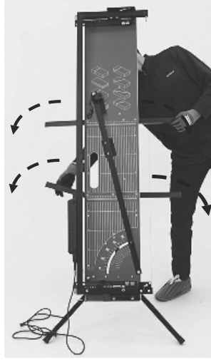
7. Attach Side Support Panels
