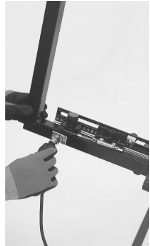
8. Connect Power Cable to Bow
