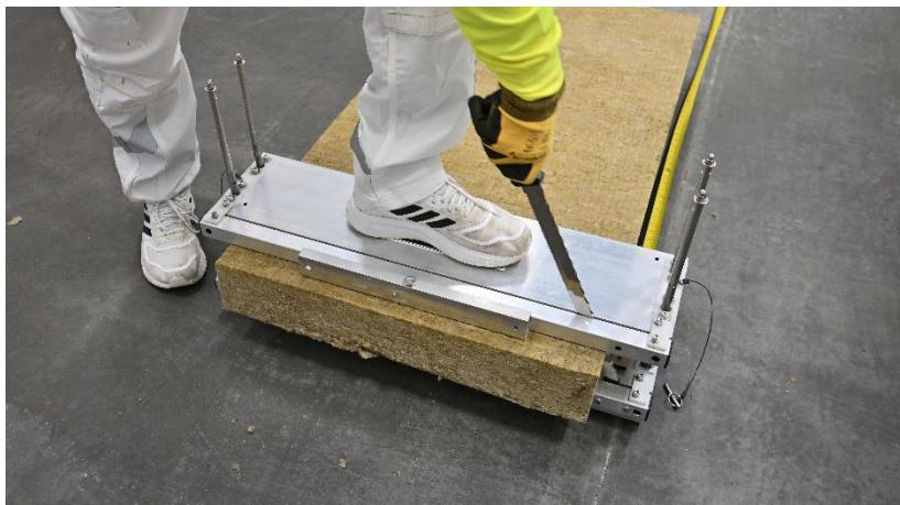
Step down on the top plate to compress the insulation material using the natural weight of your body.
