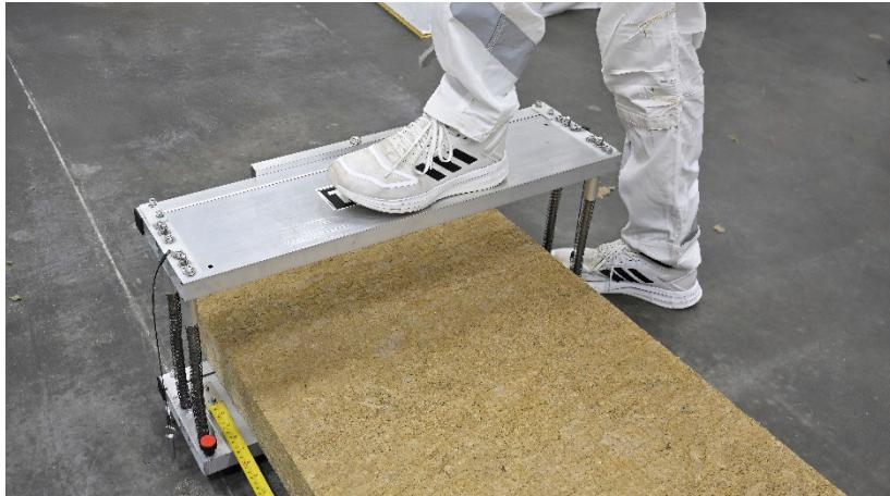
Place your preferred foot in the center of the top plate of the FINSULCUT™-100 Insulation Cutting Station.
