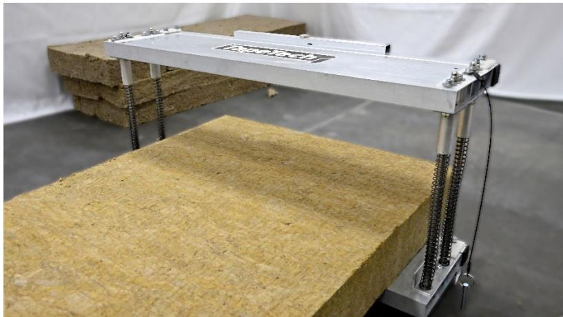
Insert the insulation material between the upper and lower plates of the FINSULCUT™-100 Insulation Cutting Station. Using the built-in measuring tape – which is calibrated to the cutting slot of the station – move the material to the required measurement.
